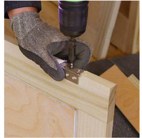
Plan for adjustability. Place the hinges with the horizontal holes on the door and the vertical holes on the cabinet, and you’ll have some room for adjusting.
