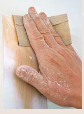
Proper technique. It's easier to control the work if you sand by hand. Fold the sheet into thirds, and hold it between your pinky and ring finger to keep it from sliding around.
