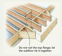
ful here. After the rim joists are in place, install the blocking, squash blocks, and any necessary cantilever reinforcements (sidebar above).
