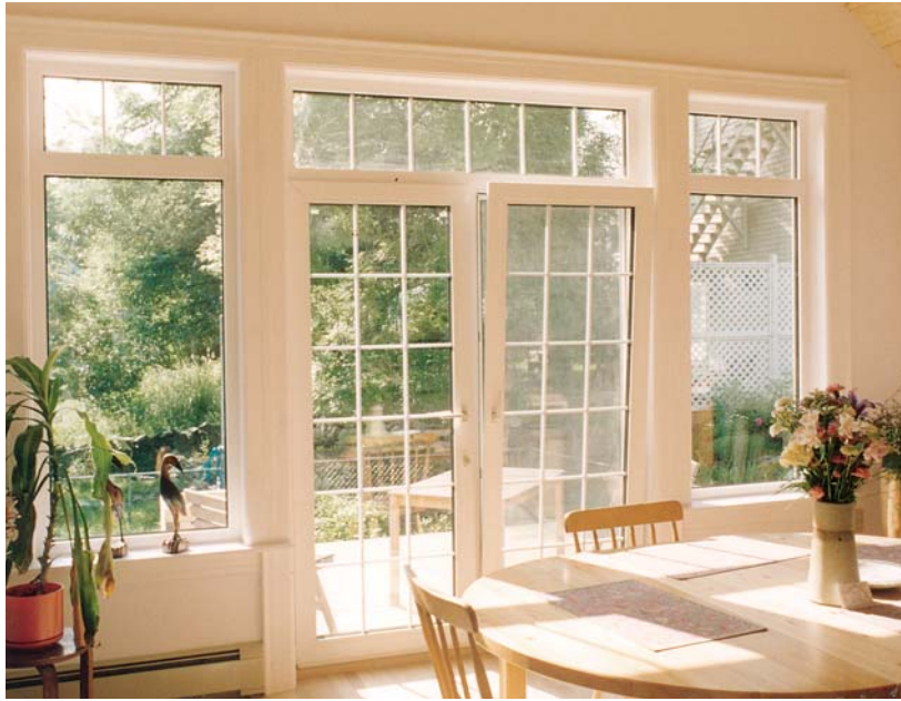
THESE DOORS TILT IN AT THE TOP and also open conventionally. The multipoint locking system secures the entire door perimeter, ensuring a tight seal and giving protection from air, water, and intruders.
