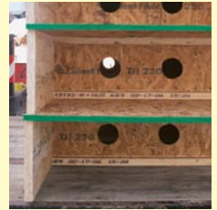
Floor panels are built in a factory setting. Trained crews assemble each panel on flat, square framing tables to maximize production speed and quality control.
