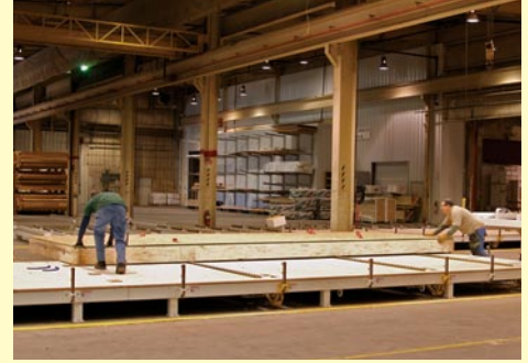
Floor panels are built in a factory setting. Trained crews assemble each panel on flat, square framing tables to maximize production speed and quality control.
