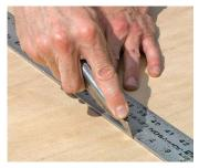
1 Cut before sawing. Scribing the cutline with a utility knife can help to reduce tearout when making finish cuts.
