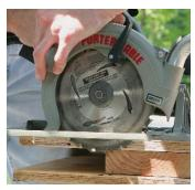
Adjust cutting depth. The blade should extend no more than ¼ in. below the bottom of the panel.
