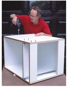
Joining door and box. With the cup portion of the hinge secured to the door, the author affixes the hinge arm into the predrilled holes in the box and adjusts the final position of the door.
