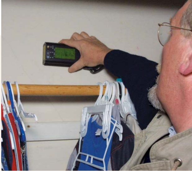
X-ray test tells you where the lead is. The black pointed lines on the view screen of this X-ray device indicate that the plaster walls in this closet are covered with lead-based paint.
