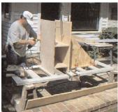
Matching sawhorses support the workbench top, which is an old door with its panels removed. Along with various L-shaped jigs, the open-paneled door facilitates clamping boards on edge and vertical assemblies. Because the old door was salvaged, it's left outside standing on its edge next to the sawhorses at the end of the workday.
