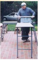
A tablesaw in a portable stand with an upgraded fence and outfeed extension adds safety, stability and accuracy. When possible, orient the tablesaw and miter saw so that when you're cutting, the stock runs in the same direction. Also, be aware of the tablesaw's need for infeed and outfeed space.
