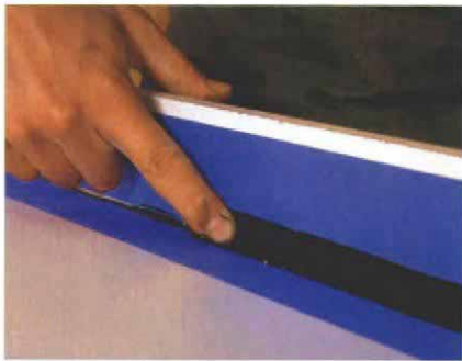
Silicone caulk seals the mold seams and creates an eased counter edge. Tape defines the area to be caulked (top photo); a moistened finger creates the concave profile (bottom photo).
