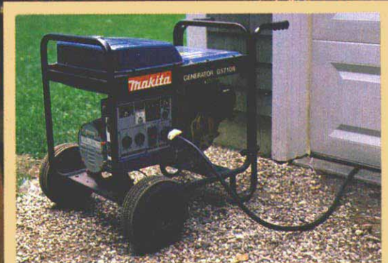
Safe backup power. An electric-start generator can power essential household circuits when the utility's power goes out. Generators should not be run in spaces that are enclosed and unventilated.
