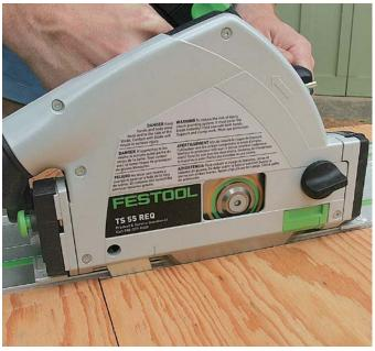
no chipping. The improved quality of cut is especially noticeable on materials prone to chipping, such as melamine. Track saws also can plunge cut, which is more difficult and less accurate with a traditional circular saw.
