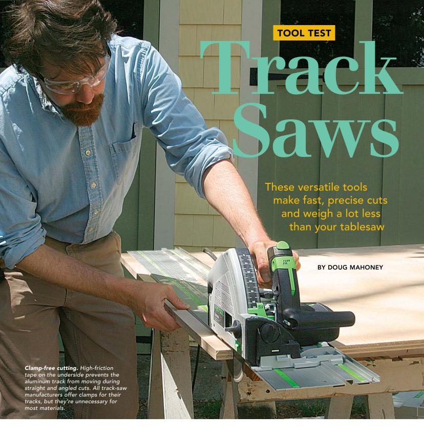
ombining a plunge-cutting circular saw with an aluminum guide rail, track saws have gone from obscure woodworking tools to common job-site problem solvers in less than 10 years. Their unsurpassed accuracy, ease of use, and clean cuts make them perfect for cutting everything from veneer plywood for cabinets and built-ins to plywood and OSB for wall and floor sheathing. Track saws are also great for trimming doors and cutting off overhanging deck boards.
