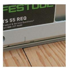
**Plunge cuts are accurate.** All the saw motors plunge by way of a spring-loaded hinge, so you have to push down on the handle to make a cut. This makes plunge and stopped cuts easy and accurate. Marks on the blade housing show where the blade is positioned within the housing.
