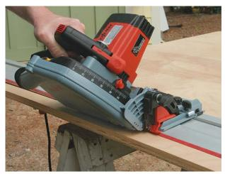
**Bevel cuts are easy.** Unlike with a conventional circular saw, the path of the blade isn't altered when a track saw is set to make a beveled cut. This makes a track saw the perfect tool for mitered corners on tapered columns, range hoods, and built-in cabinets made from sheet goods.
